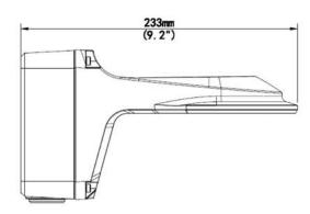
Junction Box portion contains two down facing 3/4" Conduit threaded fittings, along with an access hole in the back for cable passage if needed.
