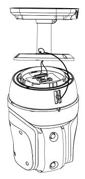
3 Line up the mold lines and assemble main body to mount adaptor and turn it..
