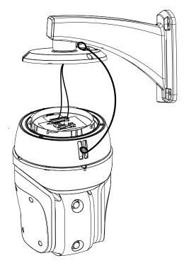
3 Line up the mold lines and assemble main body to mount adaptor and turn it.
