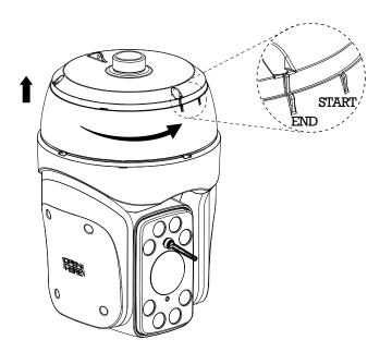
(5) Assemble the main both with the camera mount adaptor with the 3 screws. (Hexagon wrench screw M5×25).
