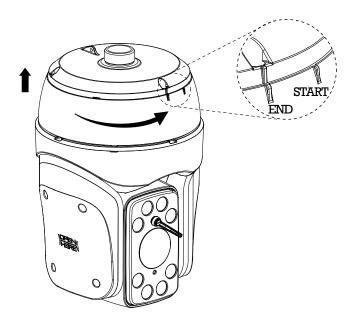
(4) Assemble the main both with the camera mount adaptor with the 3 screws. (Hexagon wrench screw  $M5 \times 25$ ).
