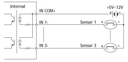
Before connecting sensors, check driving voltages and output signal types of the sensor Since output signal types of the sensors are divided into Open Collector type and Voltage Output type in general, the wiring must be done properly after considering those types.
