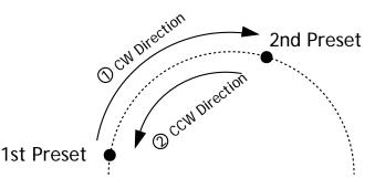
In case that the preset assigned as the 1st point and the preset assigned as the 2nd point are same, the camera turns on its axis by  $360^{\circ}$  in CW(Clockwise) direction and then it turns back on its axis by  $360^{\circ}$  in CCW(Counterclockwise) direction. The Swing speed is defined from  $10^{\circ}$ /sec to  $180^{\circ}$ /sec.
