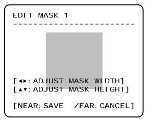
Adjusts the mask size. Use the joystick or the arrow button of your controller to adjust mask size.
