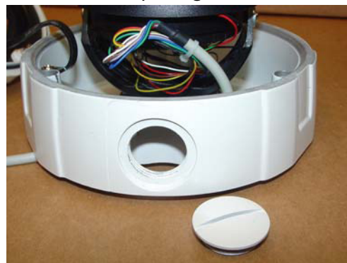
Conduit Opening (If Needed)
